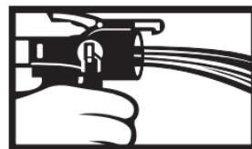
5. Select and insert firmly an Anti-Crossover Nozzle into the INSTA-FLO™ dispenser. Be sure the dispenser clips the nozzle firmly in place.
