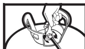
The wrench is intentionally designed to warp or bend if excessive pressure is applied.
